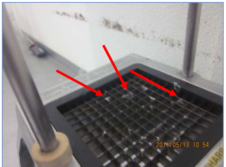
A1d. Produce dicer showing lack of proper washing as evidenced by leftover food debris on lower part.
